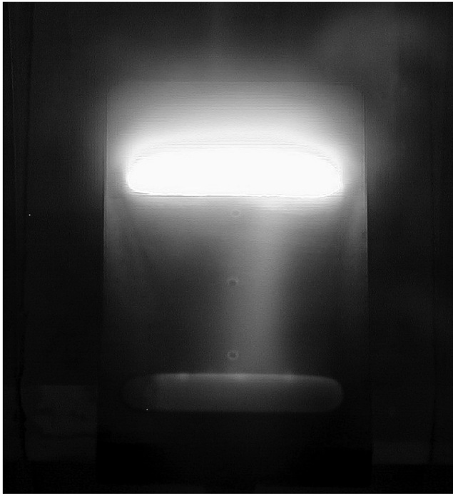
Fig. 7 100 mA, 140 W discharge, point A in Fig. 6. View is from location downstream and above plate. Flow is from top-to-bottom, cathode is at top of image.
